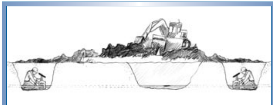
Figure 5. Conventional method for repairing large-diameter distribution lines.
