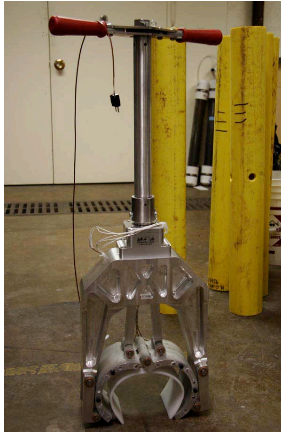
Figure 12: Final test tool with repair patch
