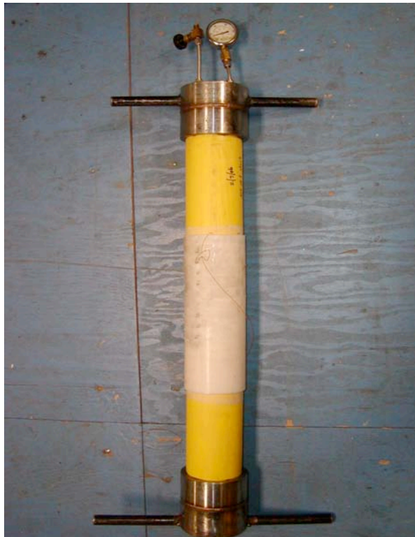
Figure 43: Closed system overlapping full-wrap gel film patch held at R^\circ & 200 psi for > 5 months without any loss in pressure
