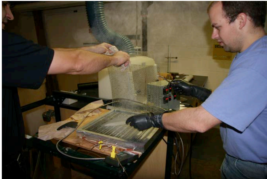
Figure 37: Swelling process used to fabricate a large PE gel film patch
