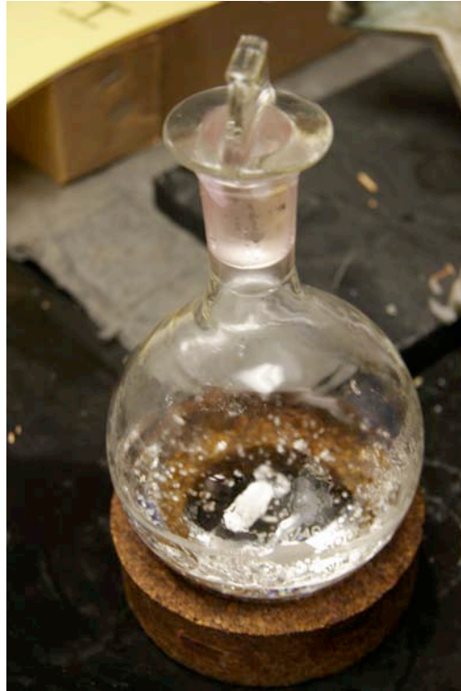
Figure 15: UHMWPE powder dissolved in heated solvent
