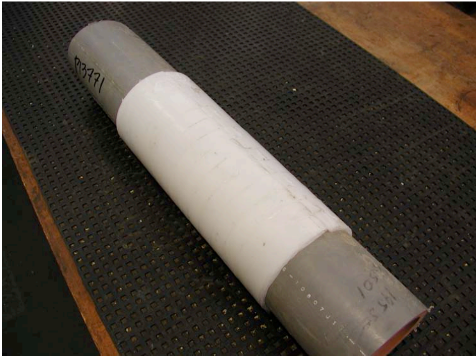
Figure 51: Overlapping full-wrap PE gel film patch successfully bonded to oxidized 4" IPS Aldyl-A pipe during demonstration for Sempra Energy
