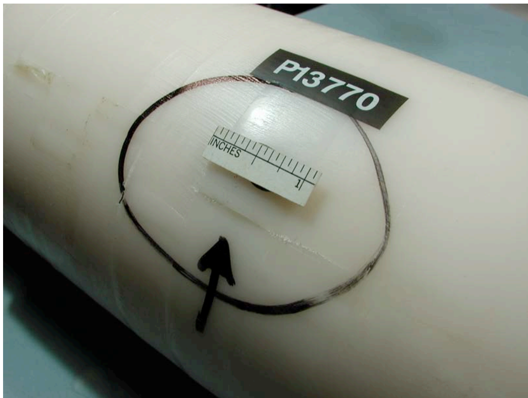
Figure 44: Photo of HDPE patch material failure at the 25-year mark during accelerated age testing
