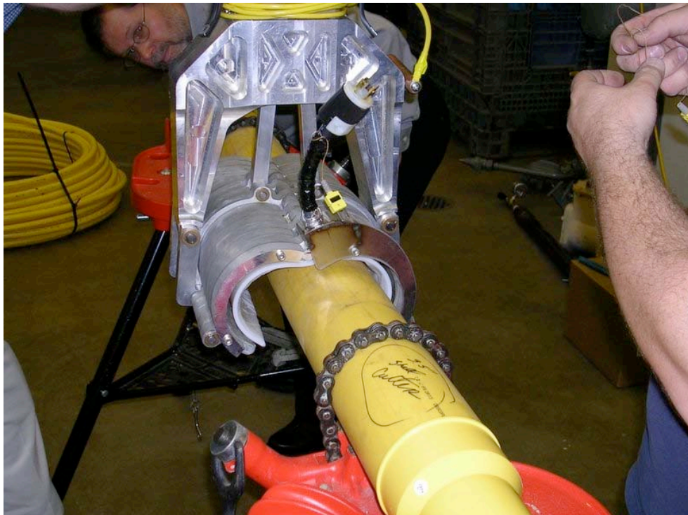
Figure 49: Engineer prototype with PE gel film repair patch being applied to damaged 4-inch MDPE pipe
