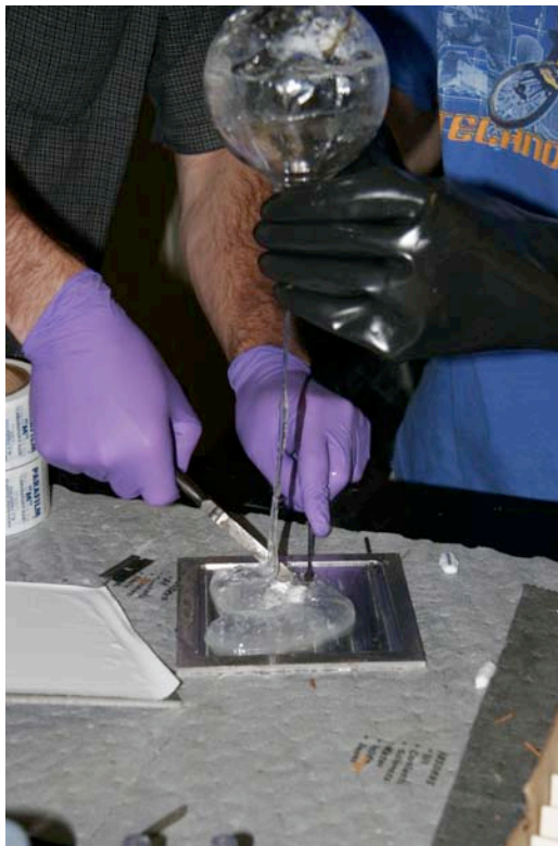
Figure 16: Dissolved UHMWPE pressed into a sheet
