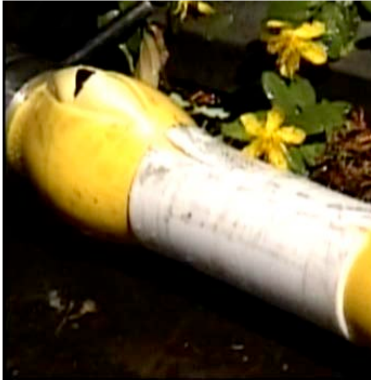
Figure 42: Quick burst test with overlapping full-wrap gel film patch shows successful bond & pipe failure below the patch at 600 psi
