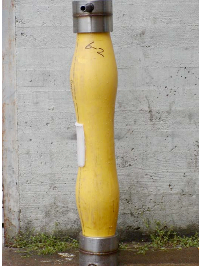
Figure 27: Pipe sample repaired with half patch showing hoop stress reinforcement
