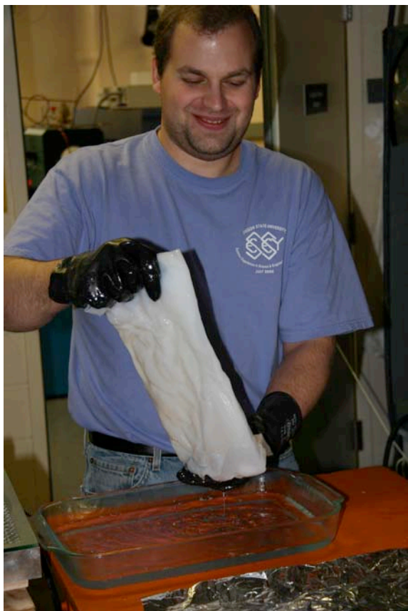
Figure 38: Photo of the final large PE gel film patch after the swelling process
